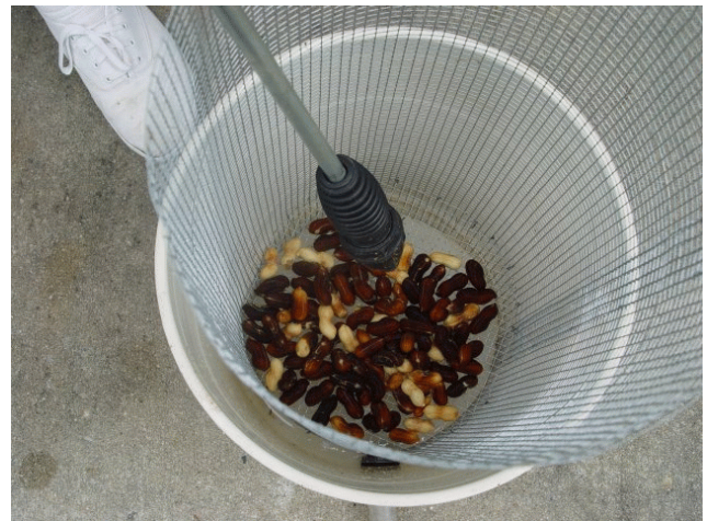
Figure 2. Pods blasted in basket with turbo nozzle.
